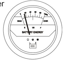
**⚠ WARNING: Never use lifter if battery energy is lower than 20% of capacity.**
